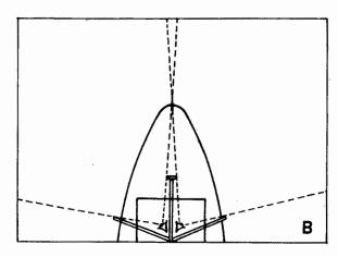
Figure 4. Limitation of the field of view by boards for one (A) or two (B) observers placed on the cabin roof of the boat.
