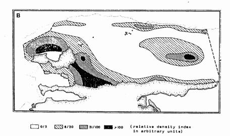
Figure 5. Example of acoustic survey mapping (from Gerlotto pers. com.) (A) survey design, (B) density mapping
